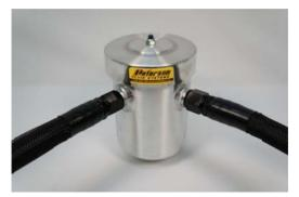
Watson Racing, LC 18703 Dix Toledo Rd Brownstown, MI 48193 855-928-7223  Remove passenger side PCV fitting in valve cover. Replace with new black straight PCV fitting supplied in kit.
